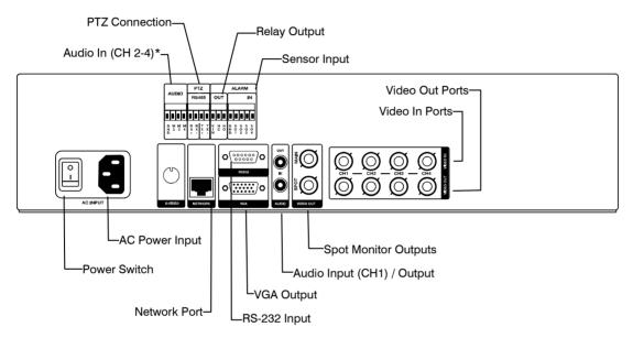
\* Audio In (CH 2-4) only available on Rev B models. (see serial number label on DVR for Rev B indication) Models earlier than Rev B support 1 CH of Audio In
