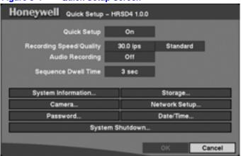
The Quick Setup screen allows you to set up the most commonly used features of your DVR. Use the arrows to move through the options. Press (#) to make your selections.
